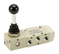
Metal Work pneumatic manual valve, 5-port (4-way), 3-position, center closed, 90 deg hand lever, detented, 1/8in female NPT inlet(s), 1/8in female NPT outlet(s), 1/8in female NPT exhaust(s), Cv=0.55.
