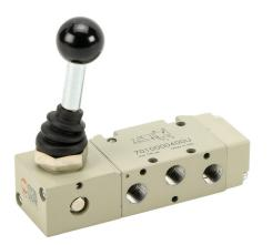
Metal Work pneumatic manual valve, 5-port (4-way), 2-position, 90 deg hand lever, detented, 1/8in female NPT inlet(s), 1/8in female NPT outlet(s), 1/8in female NPT exhaust(s), Cv=0.55.
