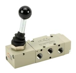
Metal Work pneumatic manual valve, 5-port (4-way), 2-position, 90 deg hand lever, spring return, 1/8in female NPT inlet(s), 1/8in female NPT outlet(s), 1/8in female NPT exhaust(s), Cv=0.55.
