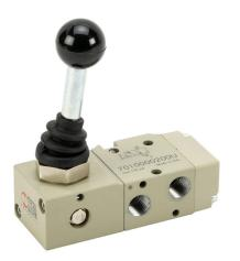
Metal Work pneumatic manual valve, 3-port (3-way), 2-position, 90 deg hand lever, detented, 1/8in female NPT inlet(s), 1/8in female NPT outlet(s), 1/8in female NPT exhaust(s), Cv=0.55.
