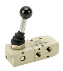
Metal Work pneumatic manual valve, 3-port (3-way), 2-position, N.C., 90 deg hand lever, spring return, 1/8in female NPT inlet(s), 1/8in female NPT outlet(s), 1/8in female NPT exhaust(s), Cv=0.55.
