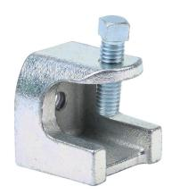
Minerallac screw-on beam clamp, 525 lbs. Package of 6. For use with flanges up to 3/4in and 5/16-18 threaded rod.
