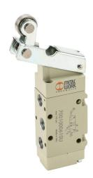
Metal Work pneumatic mechanically operated directional control valve, 5-port (4-way), 2-position, unidirectional roller lever, spring return, 1/8in female NPT inlet(s), 1/8in female NPT outlet(s), 1/8in female NPT exhaust(s), Cv=0.55.
