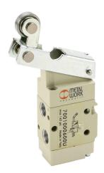
Metal Work pneumatic mechanically operated directional control valve, 3-port (3-way), 2-position, N.C., unidirectional roller lever, spring return, 1/8in female NPT inlet(s), 1/8in female NPT outlet(s), 1/8in female NPT exhaust(s), Cv=0.55.
