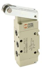
Metal Work pneumatic mechanically operated directional control valve, 5-port (4-way), 2-position, roller lever, spring return, 1/8in female NPT inlet(s), 1/8in female NPT outlet(s), 1/8in female NPT exhaust(s), Cv=0.55.
