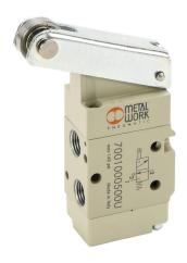
Metal Work pneumatic mechanically operated directional control valve, 3-port (3-way), 2-position, N.C., roller lever, spring return, 1/8in female NPT inlet(s), 1/8in female NPT outlet(s), 1/8in female NPT exhaust(s), Cv=0.55.
