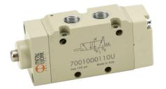
Metal Work pneumatic mechanically operated directional control valve, 5-port (4-way), 2-position, metal plunger, spring return, 1/8in female NPT inlet(s), 1/8in female NPT outlet(s), 1/8in female NPT exhaust(s), Cv=0.55.
