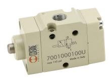
Metal Work pneumatic mechanically operated directional control valve, 3-port (3-way), 2-position, N.C., metal plunger, spring return, 1/8in female NPT inlet(s), 1/8in female NPT outlet(s), 1/8in female NPT exhaust(s), Cv=0.55.
