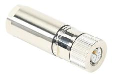
Murrelektronik connector, field-wireable, 5-pin M12 axial female L-coded, accepts cable diameter size 9-13mm, 16-14 AWG, pushlock spring clamp connection, IP65.
