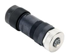
Murrelektronik field wireable connector, 5-pin M12 axial female L-coded, accepts cable diameter size 8-13mm, 14 AWG, screw terminal connection, IP67.
