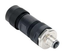
Murrelektronik connector, field-wireable, 5-pin M12 axial male L-coded, accepts cable diameter size 8-13mm, 14 AWG, screw terminal connection, IP67.
