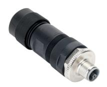
Murrelektronik field wireable connector, 5-pin M12 axial male L-coded, accepts cable diameter size 8-13mm, 14 AWG, screw terminal connection, IP67.
