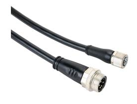
Murrelektronik adapter cable, M12 axial female L-coded to 7/8in axial male, 5-pole, 63 VDC, 12A, 16 AWG, PUR jacket, black, 6.5ft/2m cable length, IP67.
