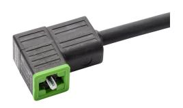
Murrelektronik valve actuator cable, 9.4mm DIN style Form CI molded connector to 4-wire pigtail, 230 VAC/VDC, 18 AWG, polyurethane jacket, IP67, 16.4ft/5m cable length.
