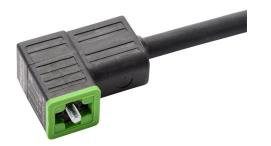
Murrelektronik valve actuator cable, 9.4mm DIN style Form CI molded connector to 4-wire pigtail, 230 VAC/VDC, 18 AWG, polyurethane jacket, IP67, 16.4ft/5m cable length.
