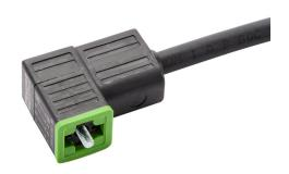
Murrelektronik valve actuator cable, 9.4mm DIN style Form CI molded connector to 4-wire pigtail, 230 VAC/VDC, 18 AWG, polyurethane jacket, IP67, 9.8ft/3m cable length.
