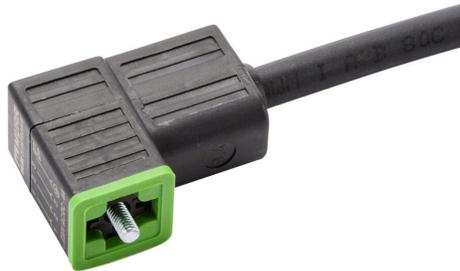
Murrelektronik valve actuator cable, 9.4mm DIN style Form CI molded connector to 4-wire pigtail, 230 VAC/VDC, 18 AWG, polyurethane jacket, IP67, 9.8ft/3m cable length.
