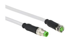
Murrelektronik connection cable, M8 axial male A-coded to M8 axial female A-coded, 4-pole, 50 VAC/60 VDC, 4A, 24 AWG, PVC jacket, gray, unshielded, 16.4ft/5m cable length, IP65 IP66K IP67 IP68, sensor & signal.
