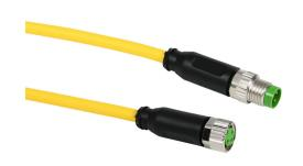
Murrelektronik connection cable, M8 axial male to M8 axial female, 3-pole, PUR jacket, yellow, 9.8ft/3m cable length, IP65 IP66K IP67.
