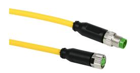
Murrelektronik connection cable, M8 axial male to M8 axial female, 3-pole, PUR jacket, yellow, 9.8ft/3m cable length, IP65 IP66K IP67.
