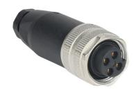
Murrelektronik connector, field-wireable, 7/8in - 16 UN2 axial female with female threads, accepts cable diameter size 6-8mm, 16 AWG, screw terminal connection, IP67.
