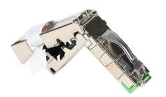
Murrelektronik Cat5e Ethernet connector, field-wireable, 8-pin RJ45 90 degree male heavy duty, accepts cable diameter size 5-9mm, 24-26 AWG, insulation displacement (IDC) connection, IP20.
