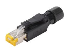
Murrelektronik Cat6a Ethernet connector, field-wireable, RJ45 8-pole Ethernet male axial, accepts cable diameter size 4.5-9mm, 26-22 AWG, insulation displacement (IDC) connection, IP20.
