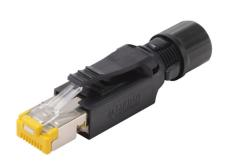
Murrelektronik field wireable connector, RJ45 8-pole Ethernet male axial, accepts cable diameter size 4.5-9mm, 26-22 AWG, insulation displacement (IDC) connection, shielded, IP20. Exceeds Category 6A specifications.
