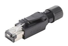
Murrelektronik Cat5e Ethernet connector, field-wireable, RJ45 4-pole Ethernet male axial, accepts cable diameter size 4.5-9mm, 26-22 AWG, insulation displacement (IDC) connection, IP20.
