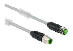
Murrelektronik connection cable, M12 axial male A-coded to M12 axial female A-coded, 8-pole, 30 VAC/VDC, 2A, 24 AWG, PUR jacket, gray, unshielded, 16.4ft/5m cable length, IP65 IP66K IP67, sensor & signal and drag chain.
