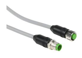
Murrelektronik connection cable, M12 axial male A-coded to M12 axial female A-coded, 8-pole, 30 VAC/VDC, 2A, 24 AWG, PUR jacket, gray, unshielded, 6.5ft/2m cable length, IP65 IP66K IP67, sensor & signal and drag chain.
