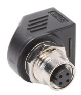
Murrelektronik field wireable Ethernet connector, M12 D-coded female 4-pole to RJ45 female Ethernet 90-degree, M12-IP68, RJ45-IP20. Mounting nut(s) included. Exceeds Category 5E specifications.
