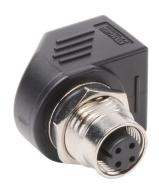
Murrelektronik bulkhead connector, field-wireable, M12 D-coded female 4-pin to RJ45 female 8-pin 90-degree, M12-IP68, RJ45-IP20.
