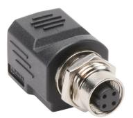
Murrelektronik bulkhead connector, field-wireable, M12 D-coded female 4-pin to RJ45 female 8-pin, M12-IP68, RJ45-IP20.
