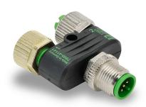
Murrelektronik T-coupler, 5-pole male M12 barrel to (2) 5-pole female M12 nuts, parallel distribution.
