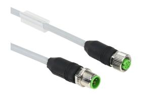
Murrelektronik connection cable, M12 axial male A-coded to M12 axial female A-coded, 5-pole, 60 VAC/VDC, 4A, 22 AWG, PUR jacket, gray, shielded, 9.8ft/3m cable length, IP65 IP66K IP67, sensor & signal and drag chain.
