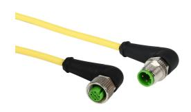
Murrelektronik connection cable, M12 right-angle male to M12 right-angle female, 4-pole, PUR jacket, yellow, 9.8ft/3m cable length, IP65 IP66K IP67.
