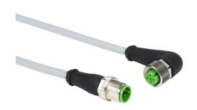
Murrelektronik connection cable, M12 axial male A-coded to M12 90-degree female A-coded, 4-pole, 250 VAC/VDC, 4A, 22 AWG, PVC jacket, gray, unshielded, 16.4ft/5m cable length, IP65 IP66K IP67, sensor & signal.
