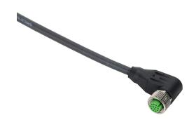
Murrelektronik connection cable, M12 right-angle female to pigtail, 12-pole, PUR jacket, black, 32.8ft/10m cable length, IP67.
