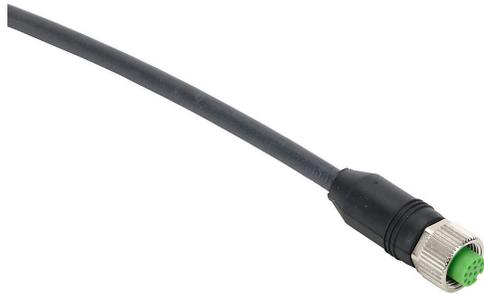
Murrelektronik connection cable, M12 axial female to pigtail, 12-pole, PUR jacket, black, 32.8ft/10m cable length, IP67.
