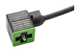
Murrelektronik valve actuator cable, 18mm DIN style Form A molded connector to 4-wire pigtail, 230 VAC/VDC, 18 AWG, polyurethane jacket, IP67, 16.4ft/5m cable length.
