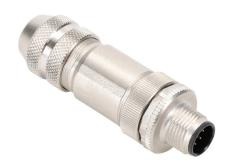
Murrelektronik connector, field-wireable, M12 barrel 8-pin male axial connection, accepts cable diameter size 6-8mm, 20 AWG, screw terminal connection, IP67.
