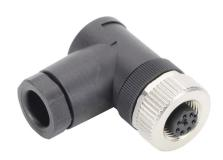
Murrelektronik connector, field-wireable, M12 nut 8-pin female right-angle connection, accepts cable diameter size 6-8mm, 20 AWG, screw terminal connection, IP67.
