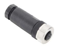
Murrelektronik field wireable connector, M12 nut 8-pin female axial connection, accepts cable diameter size 6-8mm, 20 AWG, screw terminal connection, IP67.
