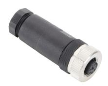
Murrelektronik connector, field-wireable, M12 nut 8-pin female axial connection, accepts cable diameter size 6-8mm, 20 AWG, screw terminal connection, IP67.
