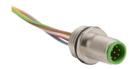
Murrelektronik bulkhead connector, M12 8-pin male to pigtail, 24 AWG, 3.2ft/1m cable length, nylon 12 conductor insulation material, IP67.
