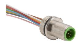
Murrelektronik bulkhead connector, M12 8-pin male to pigtail, 24 AWG, 1.6ft/0.5m cable length, nylon 12 conductor insulation material, IP67.
