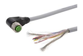
Murrelektronik connection cable, M12 right-angle female to pigtail, 8-pole, PUR jacket, gray, shielded, 16.4ft/5m cable length, IP65 IP67.
