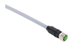
Murrelektronik connection cable, M12 axial female to pigtail, 8-pole, PUR jacket, gray, shielded, 16.4ft/5m cable length, IP67.
