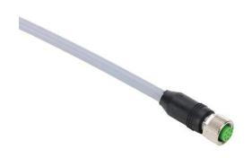
Murrelektronik connection cable, M12 axial female to pigtail, 8-pole, PUR jacket, gray, shielded, 16.4ft/5m cable length, IP67.
