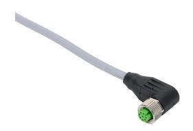
Murrelektronik connection cable, M12 right-angle female to pigtail, 8-pole, PUR jacket, gray, 16.4ft/5m cable length, IP67.
