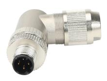
Murrelektronik connector, field-wireable, 4-pin M12 90-degree male D-coded, accepts cable diameter size 4-8mm, 26-18 AWG, push-lock spring clamp connection, IP65 IP67.
