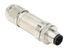
Murrelektronik connector, field-wireable, 4-pin M12 axial male D-coded, accepts cable diameter size 4-8mm, 26-18 AWG, pushlock spring clamp connection, IP65 IP67.
