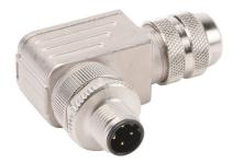
Murrelektronik connector, field-wireable, M12 D-coded 4-pole male 90-degree, accepts cable diameter size 6-8mm, 18 AWG max, screw terminal connection, IP67.
