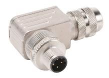
Murrelektronik field wireable Ethernet connector, M12 D-coded 4-pole male 90-degree, accepts cable diameter size 6-8mm, 18 AWG max, screw terminal connection, shielded, IP67. Exceeds Category 5E specifications.
