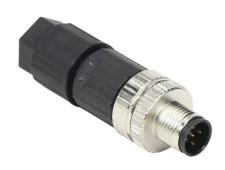
Murrelektronik connector, field-wireable, 5-pin M12 axial male A-coded, accepts cable diameter size 4-8mm, 26-18 AWG, pushlock spring clamp connection, IP65 IP67.
