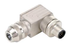
Murrelektronik connector, field-wireable, M12 barrel 5-pin male right-angle connection, accepts cable diameter size 6-8mm, 18 AWG, screw terminal connection, IP67.
