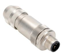
Murrelektronik connector, field-wireable, M12 barrel 5-pin male axial connection, accepts cable diameter size 6-8mm, 18 AWG, screw terminal connection, IP67.
