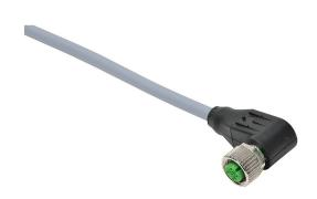
Murrelektronik connection cable, M12 right-angle female to pigtail, 5-pole, PUR jacket, gray, shielded, 32.8ft/10m cable length, IP67.
